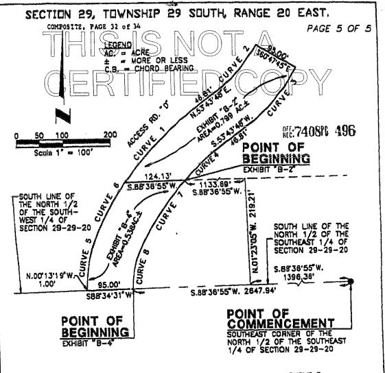
CURVE\_1 RADIUS - 897.50" DELTA = 18 27 28" ARC LENGTH = 224.70' CHORD = 223.73' C.B. = N.44'30'04"E.
